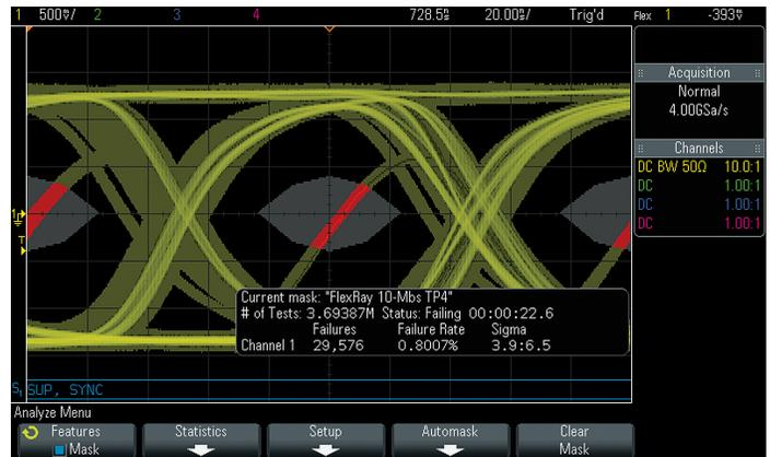
Figure 2: FlexRay “TP4” eye-diagram mask testing using a Keysight InfiniiVision 3000 X-Series oscilloscope.
