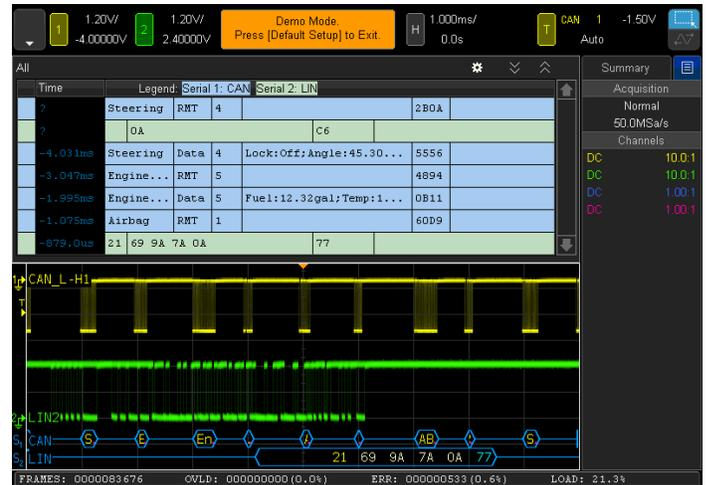
Figure 1: Capturing and decoding a CAN and LIN serial bus simultaneously on a Keysight InfiniiVision X-Series oscilloscope.
