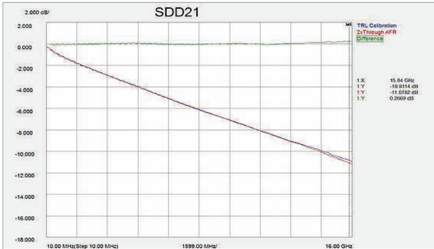
Figure 20. TRL calibration vs 2X THRU AFR
