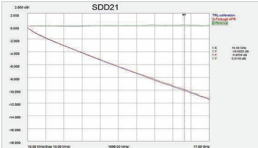
Figure 17. TRL calibration vs 2X THRU AFR
